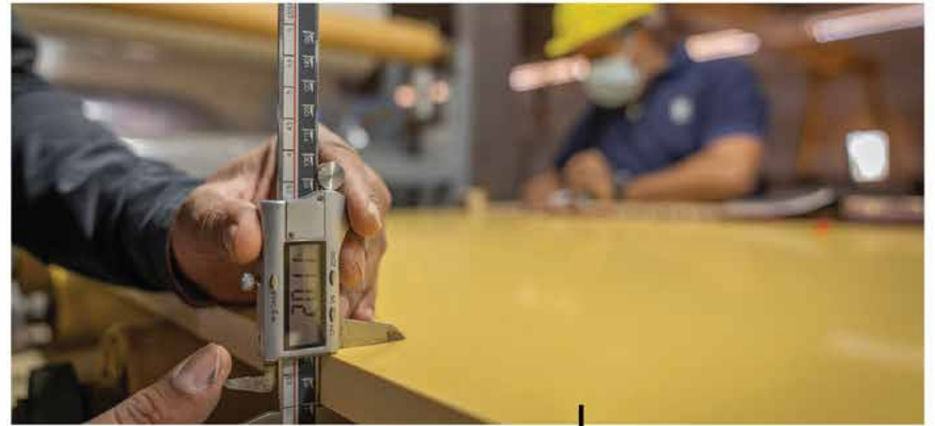
Quality Controlling & Thickness Checking
